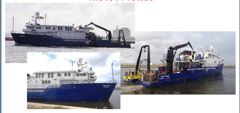
The R/V Proteus is a multi-use vessel suited for a wide variety of oceanographic research duties. The Proteus is equipped with satellite communications (voice, fax, and email), differential GPS, geophysical survey gear and large a-frames with high-speed winches for coring or geotechnical work. The Proteus is in ABS class and had an extensive technical refit in 2009 and 2014 making her ready for extended voyages. The current configuration allows up to 25 Guests /Scientists and 10 Crew.
